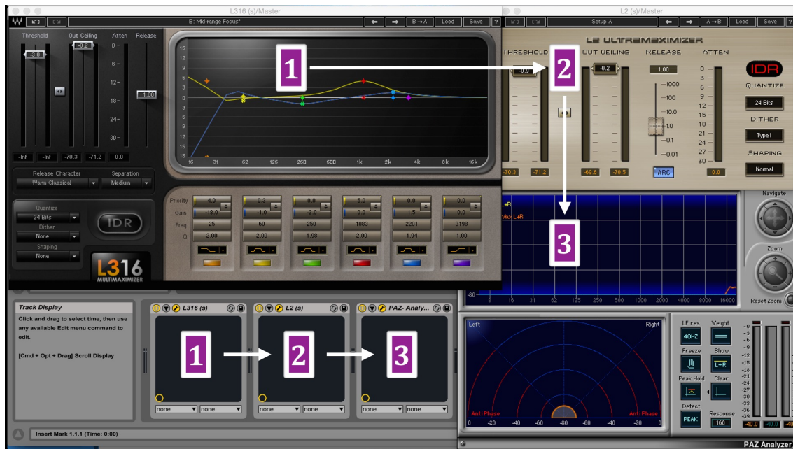
Figure 6.14.2 Screenshot showing the Waves mastering plugins used on the Master track in my Ableton Live session for Golden Sunset, Blue Rain: Field Recordings, Melodicas, Tin Whistles and Voices . The audio signal path is numbered 1 to 3.
